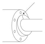
Step 1 Cutting packing at a 45° angle
